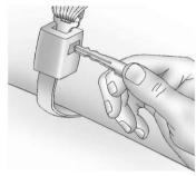
Disconnect the rear safety belt mini-latch, using a key in the slot on the mini-buckle, let the belt retract into the headliner. Stow the mini-latch in the holder located in the headliner.
